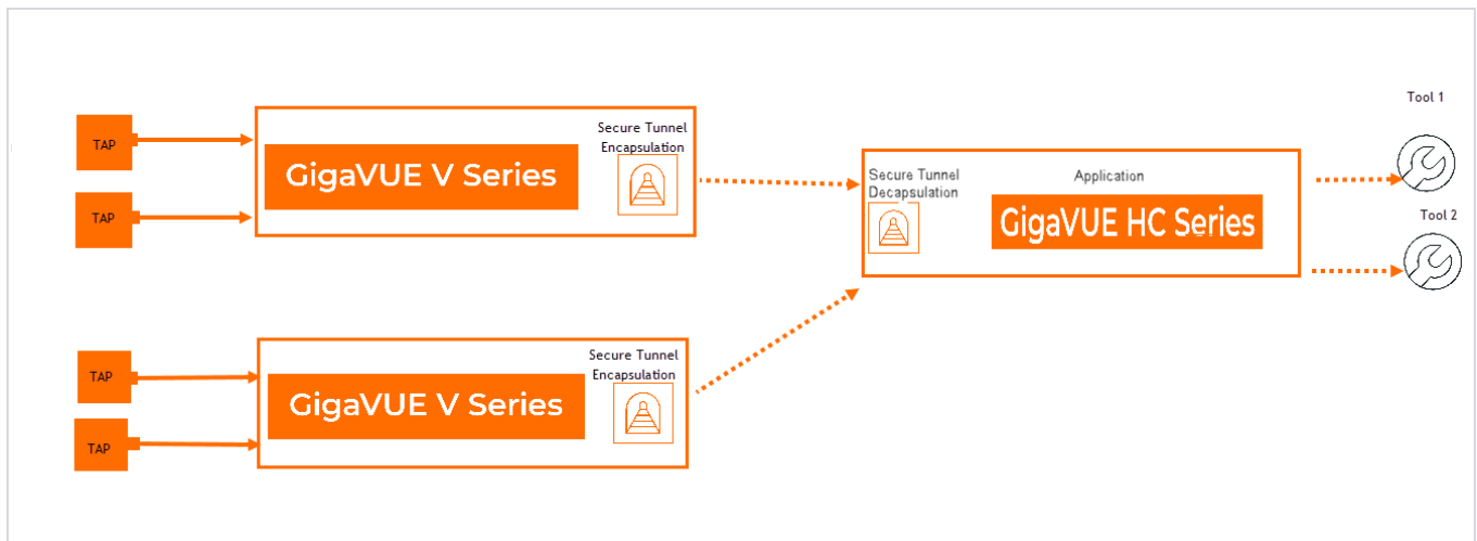
Figure 136 GigaVUE HC Series with a single IP Interface and multiple Map rules
